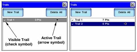
At left, Trails Menu with Trail 1 ready to record. The Active symbol shows that any travel will be recorded in this, the active trail. At right, selecting New Trail button automatically stops recording and saves
